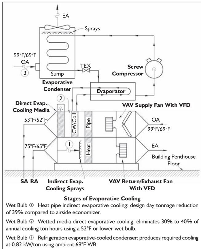
Figure 2: Evaporative cooling triple dip (design summer flow).
