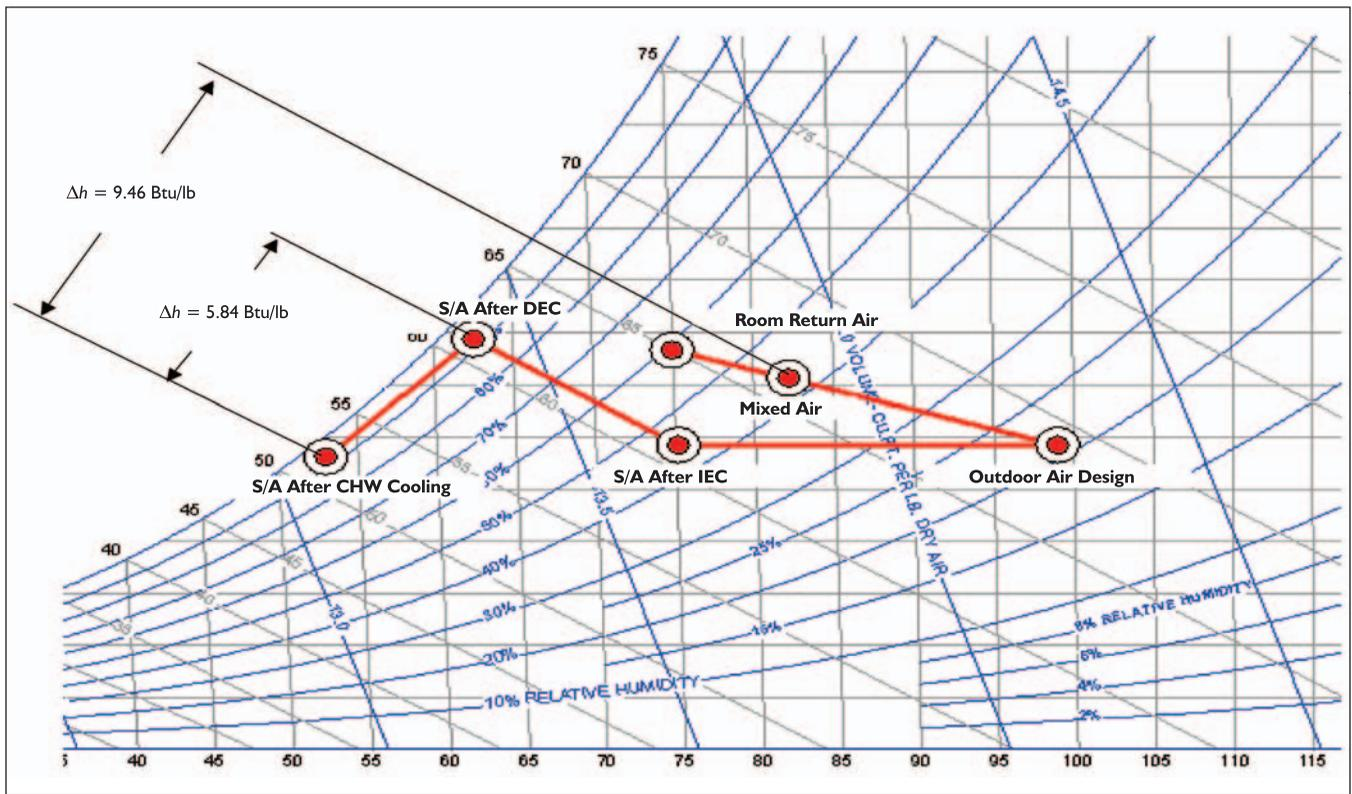
Figure 1: Santa Rosa, Calif., is a semi-arid climate where an indirect/direct evaporative cooling design may be used in summer to introduce 100% outdoor air with a 38% reduction in design day cooling tonnage.
